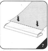
7. Peel off the adhesive paper along the edge of the base's leader roll and attach the bottom of the banner. Make sure the banner is straight. both sides.
