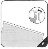
6. Finish the top by re-attaching the plastic end
