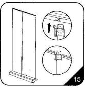
15.The plastic holder at the top of pole slips into the rear slot of the banner beam. A marker on the beam indicates the beam's centre where the
